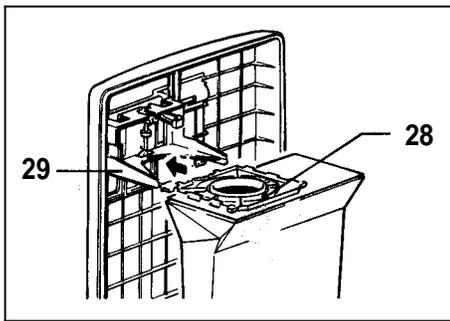
The micro hygiene filter (30) needs to be changed when it becomes clogged with dust or after approximately 20 paper bags have been used. To change the hygiene filter first remove the cover then slide the filter out at the bottom. To replace lift the lever and slide the new filter in.
